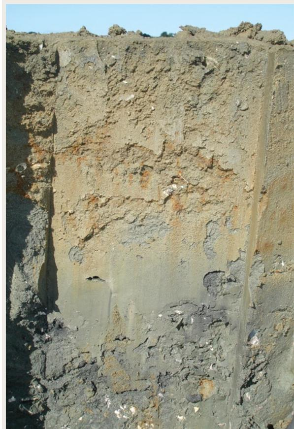
Photo: Sediment layers – by using cores and radioisotope dating to look at changes in sediment rates through time, we can determine sediment accumulation rates and relate these to human activities. (Source: ARC).
